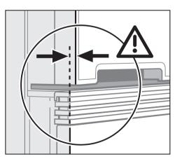
To align the door, add or remove the spacers located underneath the door latch.
